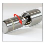
3. If using the HiTemp140-M12 data logger, screw the probe into the bottom end of the barrier lid.
