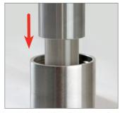
4. Slide the data logger and lid back into the barrier body and screw the lid back on tightly.
