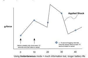
The potential to lose valuable data can be seen. This, of course, is very dependent on the applied shock duration and wave shape. It's possible for a significant shock event to occur and not even be visible in the data for the Instantaneous mode.
