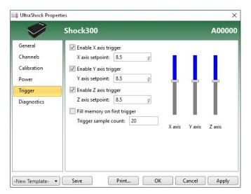
For example, if the option to fill memory is selected, then after the first trigger, all of available memory will be filled at the selected logging rate. This will consume the remainder of available storage space for the selected channel.
