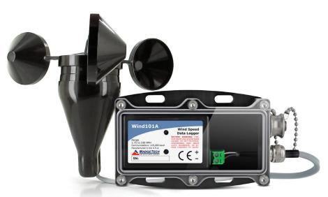
The Wind101A is a complete system to accurately measure and record wind speed. This low cost wind speed recording system comes complete with a data logger, weather-proof enclosure, a three-cup anemometer and all the necessary cabling to quickly get up-and-running. The logger can record up to 500,000 readings and the storage medium is non-volatile, solid state memory, providing maximum data security even if the battery becomes discharged.
