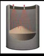
Adding an additional scanner in a wide bin provides more coverage of the material surface, ensuring greater accuracy!
