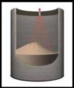
A single scanner measures in a 70° beam angle that does not cover the entire surface area.
