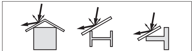
Fig. 23: Cover flat, large-area profiles with deflectors
