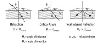
In the MA873, light from an LED passes through a prism in contact with the sample. An image sensor determines the critical angle at which the light is no longer refracted through the sample. The MA873 automatically applies temperature compensation to the measurement and converts the refractive index of the sample to Glucose concentration in units of percent (by weight).
