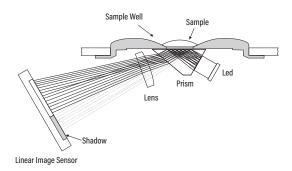
Specialized algorithms then apply temperature compensation to the measurement and convert this refractive index to: g/100 g (% by mass), g/100 mL, Specific Gravity (S.G. 20/20), or Baumé.
