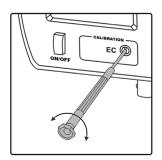
The calibration is now complete and the meter is ready for use. The instrument should be re-calibrated at least once a month, or when the probe is changed.
