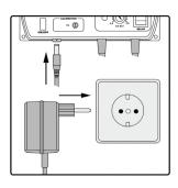
Connect the supplied 240VAC/12VDC power adapter to the meter and to the main line.
