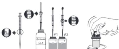
5. Remove the caps and using the second syringe add 0.5 mL of Cl-2 reagent to each cuvette. Replace the caps and swirl gently for 30 seconds.
