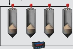
Snooper remote Modbus display located at ground level to scan level data from all sensors and automatically alternates level data from each sensor
