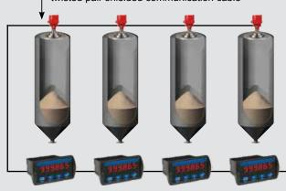
Snooper remote Modbus display located at ground level at each bin to read level data from each individual sensor
