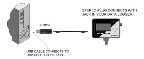
Fully insert the male connector of the IFC200 interface cable into the female receptacle of the data logger. Fully insert the female USB connector into the USB. (*Please see the Data Logger Software manual for further information.*)
