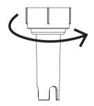
Make sure the gaskets are in place before screwing back the ring.
