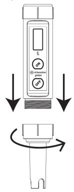
Make sure the gaskets are in place before screwing back the ring.
