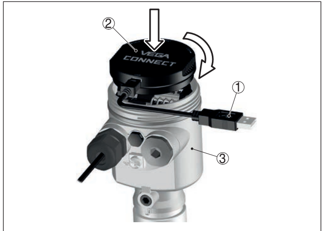
Fig. 20: Connection of the PC directly to the sensor via the interface adapter
