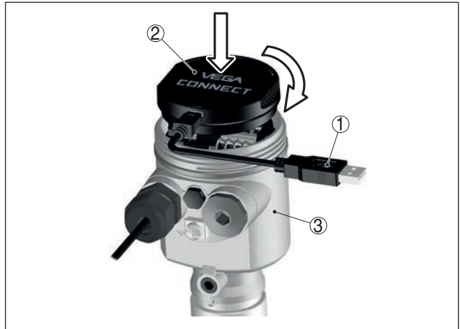
Fig. 21: Connection of the PC directly to the sensor via the interface adapter
