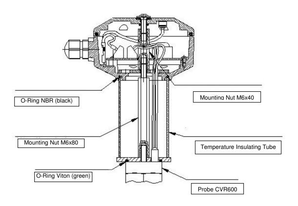
• Remote Electronics Installation (not available for dust-ex)
