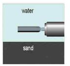
Function: A piezo system brings rod to vibrate at its resonant frequency. The vibrating system is tuned to work in water. If solid material covers the rod, it damps the vibration. An electronics circuit switches a binary output signal. When the rod gets uncovered, it starts vibrating again and the output switches back.
