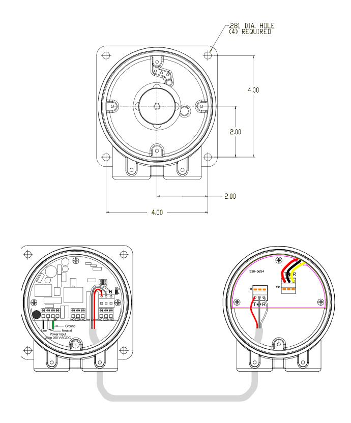
Figure 5 VR Remote Mounting Dimensions and Wiring
