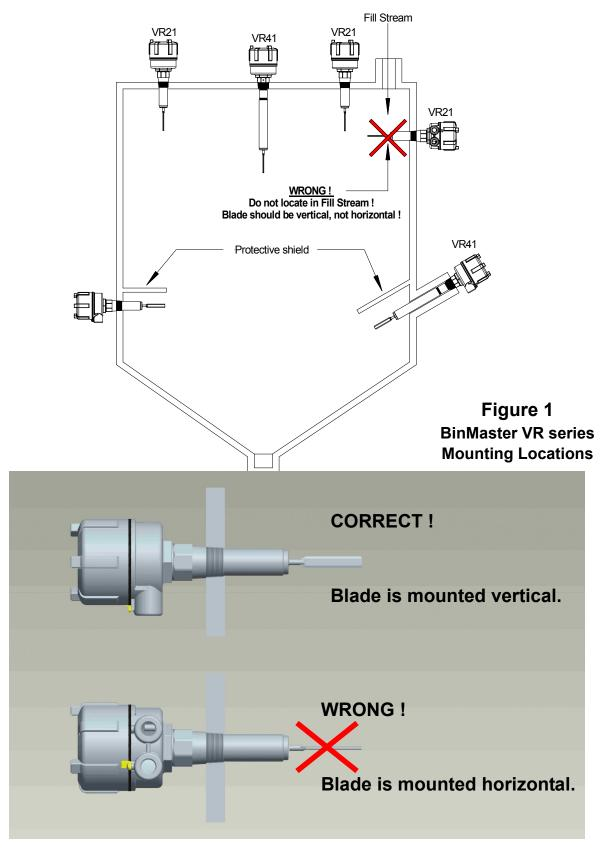
The conduit entries must always point downwards to prevent moisture from seeping inside the housing. If the housing is not in the correct position after the probe has been firmly screwed into the bin wall, proceed as follows:
