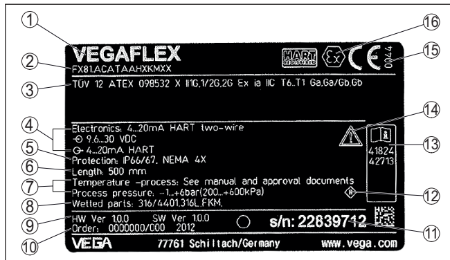
Fig. 1: Layout of the type label (example)
