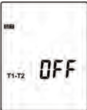
(6) Fig.6 Set T1-T2 subtraction mode.
