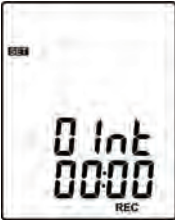
(3) Fig.3 Set interval time for data logging.
