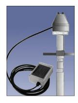
The high temperature PRO Remote capacitance probe features a heavy duty design for use in applications where the temperature exceeds 500°F (260°C). It is used to detect the level of material in a bin, tank or silo or the presence of material in a chute or spout. The probe and the electronics are separated by a cable to distance the electronics from the heat source.
