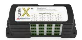
The new CurrentX Series consists of 4, 8, 12 and 16-channel, battery powered, low level DC current data loggers with a reading rate of up to 4 Hz. Improvements include the elimination of an interface cable (uses standard USB-A to Micro USB), increased memory for more readings and increased download speed.
