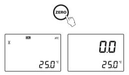
Gently absorb the ZERO water standard with a soft tissue. Use care not to scratch the prism surface. Dry the surface completely. The instrument is ready for sample measurement.
