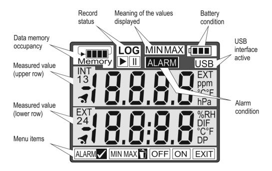
**Data memory occupancy** - this display section offers information about the current condition of the free space existing in the data memory. The blinking of the *Memory* symbol indicates that the pre-set memory occupancy limit has been exceeded. This limit can be set up in the device's configuration. Several actions can be assigned to it (optical and acoustic signalling).
