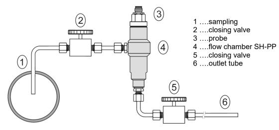
**sampling** (1) - end of the tube placed in the centre of pressure pipelines (distribution of moisture in the pipe cross-section is not homogeneous). To achieve fast response times to shorten the length of the sample tubes to a minimum (few meters).
