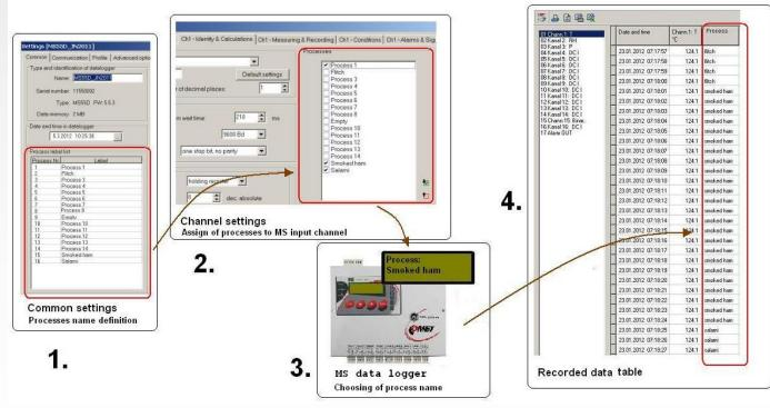
Processes allows to mark part of record with additional text. They are used to surbscribe parts of ongoing process with default text when the user needs.
