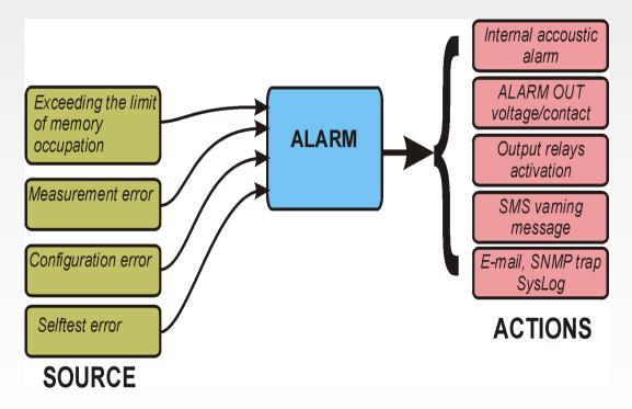
Configuration is done on global bookmark Profile. Alarms can also arised due to exceeding the limit of full memory, measurement error, MS configuration and selftest.
