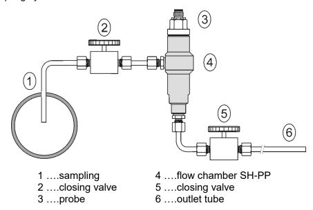
sampling (1) - end of the tube placed in the centre of pressure pipelines (distribution of moisture in the pipe cross-section is not homogeneous). To achieve fast response times to shorten the length of the sample tubes to a minimum (a few meters).
