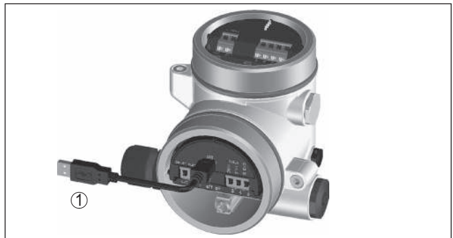
Fig. 24: Connecting the PC via USB to the Modbus electronics
