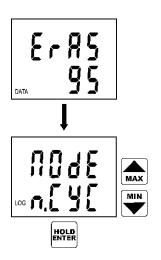
Clearing procedure is in progress. The duration is indicated by displaying of already cleared memory in % (digits 0 to 100).
