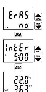
Instrument offers the possibility to clearing the instrument memory (ERAS). If you do not wish to clear the memory before new logging start, confirm selection ERAS NO by pressing the ENTER key.
