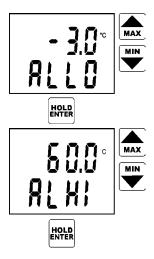
It is possible to set lower and upper limit for measured temperature. Breaking of the limit is indicated by blinking of the value on the display. Alarm activation can be disabled by setting lower alarm limit up to its maximum. This is indicated by OFF reading at the position of numeric value. Value of upper limit of the same alarm is indifferent.
