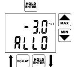
Reading ALLO indicates adjusted lower alarm limit. Set the desired value by means of the arrow keys. Press and hold the arrow key UP to make value increase fast. Press and hold the arrow key DOWN to make value decrease fast. Release the arrow key and press ENTER to confirm new limit.
