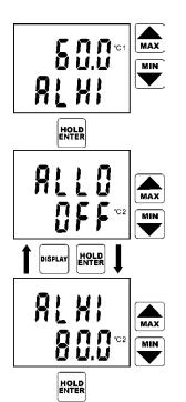
Reading ALHI indicates adjusted upper limit. Set the desired value in the same way as in above lower limit. If needed it is possible to get back to lower limit setting of the same alarm by pressing DISPLAY key. Press ENTER key to confirm new upper limit.
