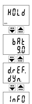
Press ENTER key to display values stored in the HOLD memory. Press DISPLAY key to display other stored values. Press MENU key to leave this mode.
