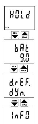
Press ENTER key to display values stored in the HOLD memory. Press DISPLAY key to display other stored values. Press ENTER key to leave this mode.
