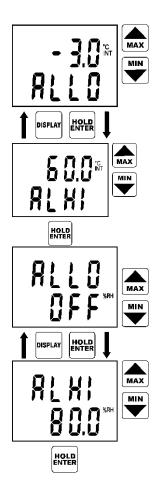
Reading ALLO indicates adjusted lower alarm limit (here air temperature). Set the desired value by means of the arrow keys. Press and hold the arrow key UP to make value increase fast. Press and hold the arrow key DOWN to make value decrease fast. Release the arrow key and press ENTER to confirm new limit.
