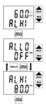
Reading ALHI indicates adjusted upper limit of the same alarm (here air temperature). Set the desired value in the same way as in above lower limit. If needed it is possible to get back to lower limit setting of the same alarm by pressing DISPLAY key. Press ENTER key to confirm new upper limit.
