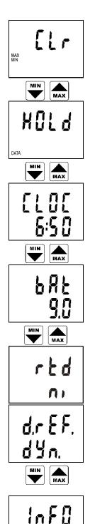
Clearing of minimum and maximum memory of temperature. Memory is cleared after pressing ENTER key. Clearing is confirmed by reading YES on the LCD lower display.
