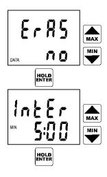
Instrument offers the possibility to clearing the instrument memory (ERAS). If you do not wish to clear the memory before new logging start, confirm selection ERAS NO by pressing the ENTER key.
