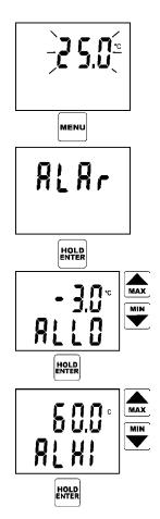
It is possible to set lower and upper limit for measured temperature. Breaking of the limit is indicated by blinking of the value on the display. Alarm activation can be disabled by setting lower alarm limit up to its maximum. This is indicated by OFF reading at the position of numeric value. Value of upper limit of the same alarm is indifferent.
