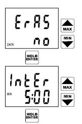
Instrument offers the possibility to clearing the instrument memory (ERAS). If you do not wish to clear the memory before new logging start, confirm selection ERAS NO by pressing the ENTER key.
