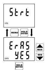
If it is needed to clear the memory before logging start, first it is necessary to select menu item logging START (symbol Strt) and confirm by pressing ENTER key.
