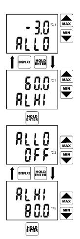
Reading ALLO indicates adjusted lower alarm limit. Set the desired value by means of the arrow keys. Press and hold the arrow key UP to make value increase fast. Press and hold the arrow key DOWN to make value decrease fast. Release the arrow key and press ENTER to confirm new limit.
