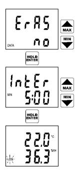
Instrument offers the possibility to clearing the instrument memory (ERAS). If you do not wish to clear the memory before new logging start, confirm selection ERAS NO by pressing the ENTER key.
