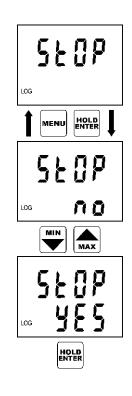
Logging stop is enabled by confirmation of menu item STOP by pressing ENTER key.
