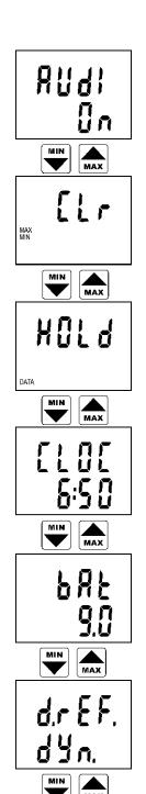
This item indicates if audio signaling of alarm indication is switched on (On) or switched off (OFF). Press ENTER key to change actual setting.
