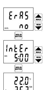
Instrument offers the possibility to clearing the instrument memory (ERAS). If you do not wish to clear the memory before new logging start, confirm selection ERAS NO by pressing the ENTER key.
