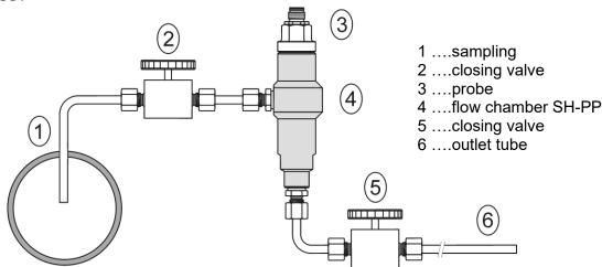
**sampling (1)** - end of the tube placed in the centre of pressure pipelines (distribution of moisture in the pipe cross-section is not homogeneous). To achieve fast response times to shorten the length of the sample tubes to a minimum (few meters).
