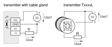
Loop resistance value Rc = R + resistance of wires shall fulfill the condition  $Rc[\Omega] < 40 \times Uss1[V] - 360$ .
