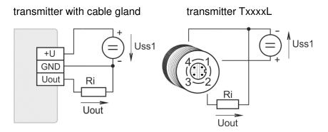
The value of the internal resistance (Ri) of the measuring instrument must be greater than 20  $k\Omega.$
