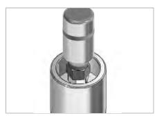
6. Tighten the Dome Nut to secure the data logger in place (fingertight).
