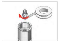
1. Wrap the provided PTFE thread sealing tape around the Fitting Body threads.
