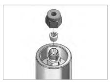
4. Insert the Compression Ferrule into the Fitting Body and hold it in place loosely with the Dome Nut.
