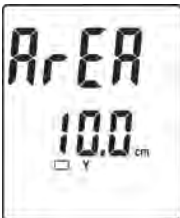
(5) Fig.5 Set Rectangle Duct Y dimension.
