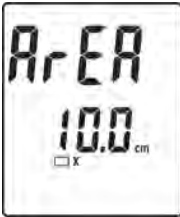
(4) Fig.4 Set Rectangle Duct X dimension.
