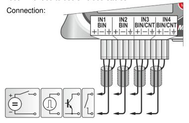
The procedure for connecting the wires to the terminals can be found in Annex 4.
