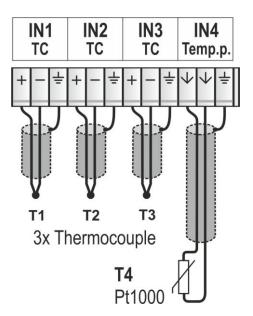
The procedure for connecting the wires to the terminals can be found in Annex 4.
