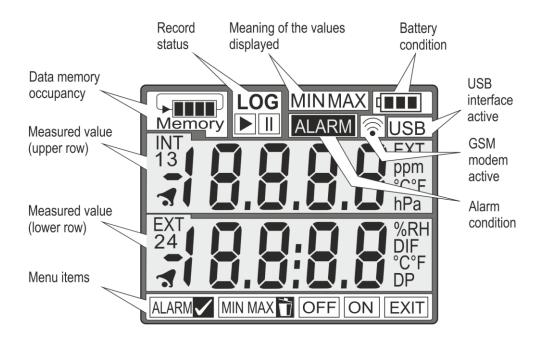
**Data memory occupancy** – this display section offers information about the current condition of the free space existing in the data memory. The blinking of the *Memory* symbol indicates that the preset memory occupancy limit has been exceeded. This limit can be set up in the device's configuration. Several actions can be assigned to it (optical and acoustic signalling, sending SMS messages).
