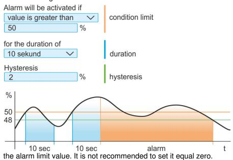
Thus, the setting for generating an alarm is completed. It remains to decide, whether the alarm should be indicated optically by means of a LED diode on the device (*Optical signalling - LED*), acoustically (*Activate internal acoustic signalling*) or by sending a alarm text message to up to four selected recipients (when alarm occurs/disappears, send SMS to selected recipients).
